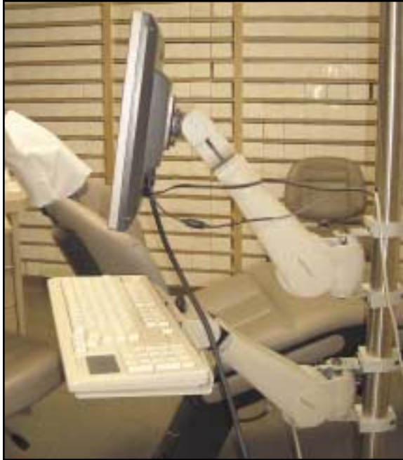
Fig. 2 Ergo arms used to attach monitor and keyboard to pole.
