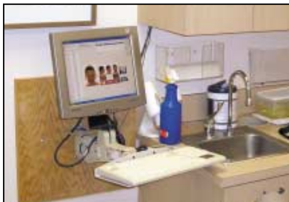
Fig. 4 Ergo arms used to attach monitor and keyboard to wall.
